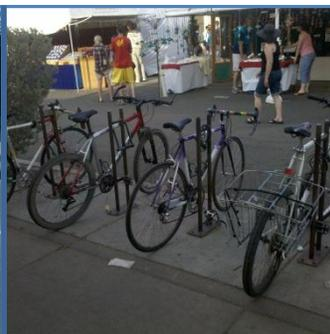
Designs can be simple with anchored rods and a supporting bar
