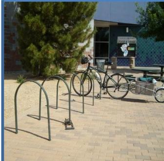
"U" racks support bike frame at 2 places and provide space for a trailer
