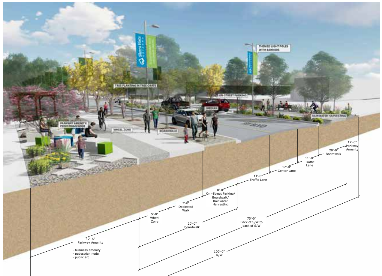
This design concept shows the key elements of the project, to include vehicle, pedestrian, and bicycle travel lanes. The streetscape amenities, such as street lights, furniture, banners, and plantings, are only representative and do not illustrate the final streetscape design concept.
