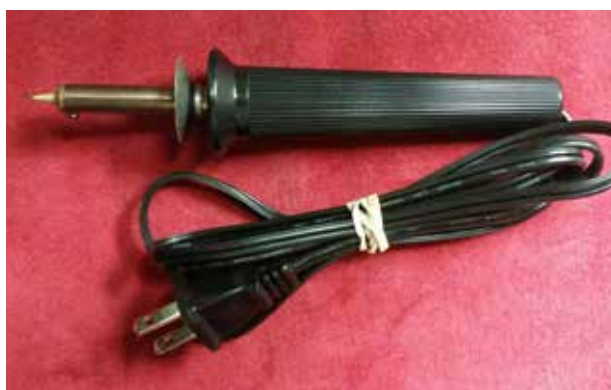
This wood burning tool, ca. 1970s, was a recent "What is It?" item.
